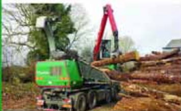
Chipping oversized log
